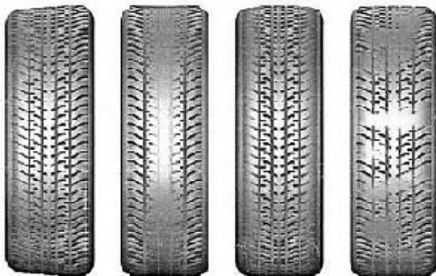
Alignment Problem Over Inflated Under Inflated Failed Strut or Shock
